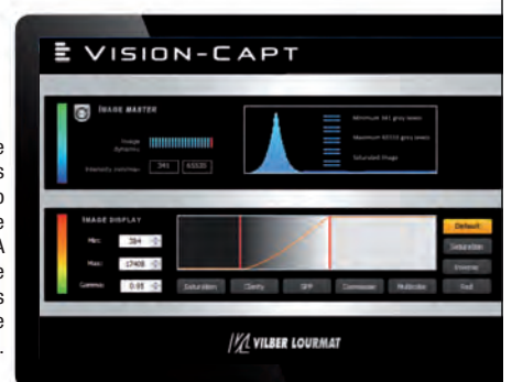
Fig.8: The Image Master Assistant is a powerful tool to control your sample image quality. A modification of the image display does not modify the Image Master data.
